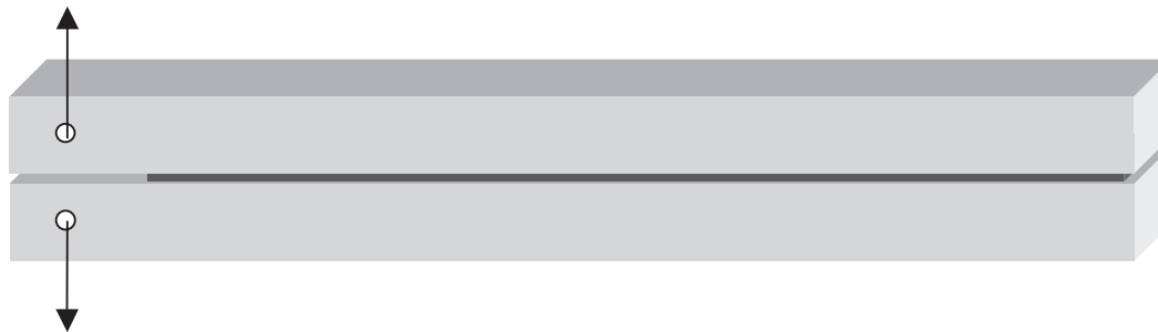
FIGURE 27.3. Diagram of an ASTM D3433 double cantilever beam specimen. The load is usually applied by attaching a fixture to holes located near the front of the specimen. In general, the initial portion of the specimen is not bonded in order to provide an initial crack.
