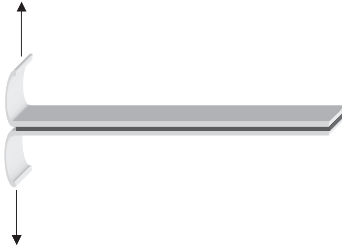
FIGURE 27.2. Diagram of an ASTM D1876 T-peel specimen.
