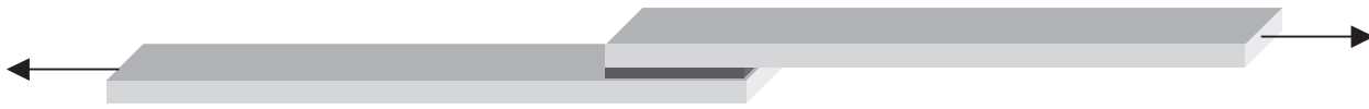
FIGURE 27.1. Diagram of an ASTM D1002 lap shear specimen. The adherends are usually 2.54 cm wide and 10.16 cm long. The thickness of the adherend depends upon the adherend material. If the adherend is aluminum, that thickness is usually 0.16 cm thick.
